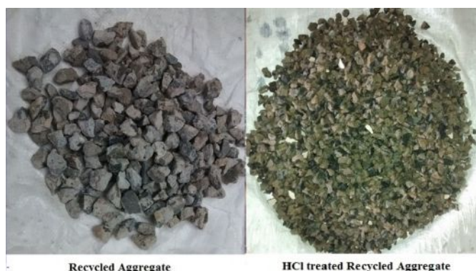
Fig. 1. Recycled aggregates before and after treatment
